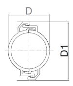
D – nominal diameter [mm]D1 – outer diameter [mm]L – length = 150mm
